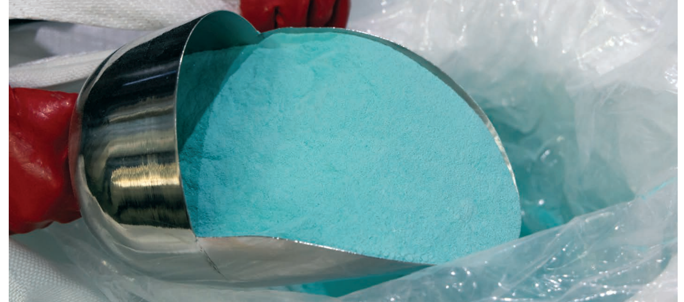
Nickel sulfate from SungEel HiTech Co., a company that specializes in recycling lithium-ion batteries in Gunsan, South Korea. SungEel collects old and defective cells from automakers and some of the country's biggest battery makers, including LG Energy Solution, and has the capacity to extract about 4,400 metric tons of nickel and cobalt annually.
