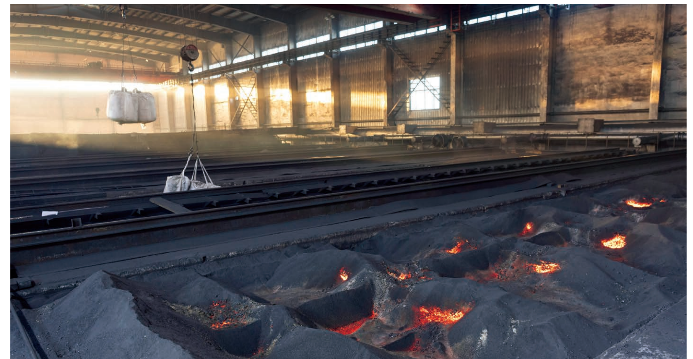
This photo taken on Dec. 8, 2022 shows the graphitization process of anode materials for lithium-ion batteries at a workshop of a company in Hegang City, northeast China's Heilongjiang Province.
